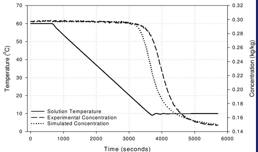
**Figure 2:** Solution temperature, experimental and simulated solution concentration for 1°C/min process runs.
