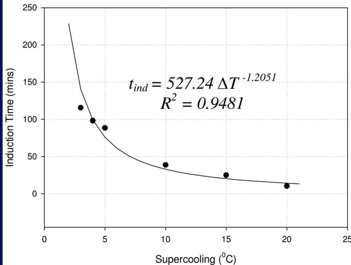
**Figure 1:** Induction times versus degree of supercooling, measured using FBRM<sup>®</sup> probe.
